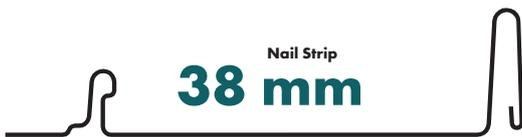
This system creates a durable sealed weather-tight joint, suitable for both cladding and roofing applications.
