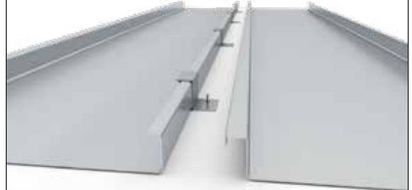
Clip hooks are fixed to the underlap of the male edge and fastened to the substrate prior to joining the adjacent female edge.
