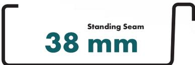
Standing Seam works by using concealed clips to secure the panel to the sub-structure which is then overlapped with an adjacent panel. These panels are then crimped together using specialised tools to create a strong sealed weather-tight join.
