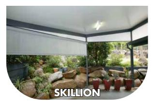
A skillion roof (single-pitch), is characterised by its single, steeply inclined plane.
