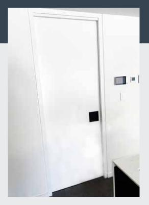
Stronger and sturdier than timber framed doors, Metroll Cavity Sliding Door Frames incorporate quality engineering with heavier gauge steel and superior reinforcing, this makes them more robust than other cavity door options.
