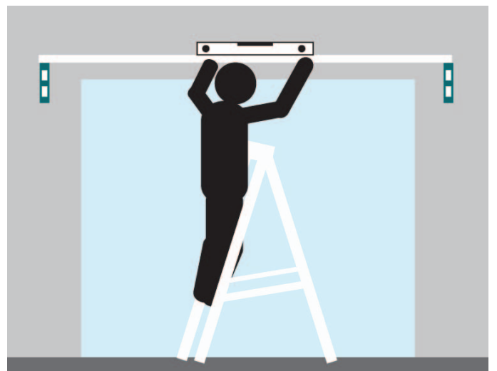
FIG.2 ENSURE BRACKETS ARE LEVEL
