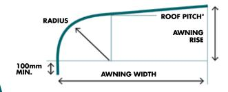
**NOTE:** Metroll takes no responsibility for variances on sheets curved from drawings. A template should be supplied to ensure accuracy. The min. recommended curving radius is 450mm.
