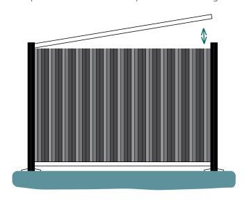
Allow for an overlap when inserting the second sheets. Refer to the below diagram:
