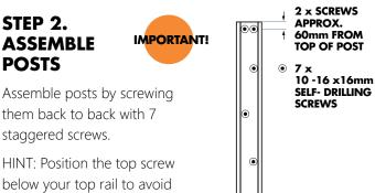
HINT: Position the top screw below your top rail to avoid catching when positioning the top rail in place.
