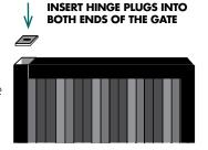
S Position the gate on the bottom hinge. Align the gate with the post and slide the top hinge into the hinge plug. Tighten the top hinge once in place.
