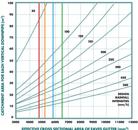
EFFECTIVE CROSS SECTIONAL AREA OF EAVES GUTTER (mm<sup>2</sup>) GRADIENT 1:500 & STEEPER
