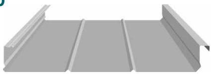
Sheet Width: 350mm Cover: 330mm Height: 44mm
